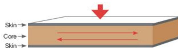
Figure 9.6 Structure of a sandwich composite [47]
