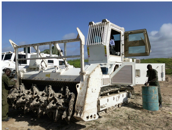
Figure 4.1 - Minewolf MW370 with a tiller attachment [21]
